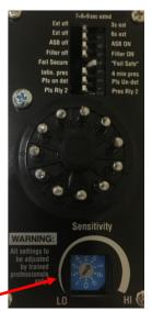
9 (highest setting). Typical applications require a setting of 3 or 4. The rotary adjustment must be set to a specific/whole number. There are no half settings.
