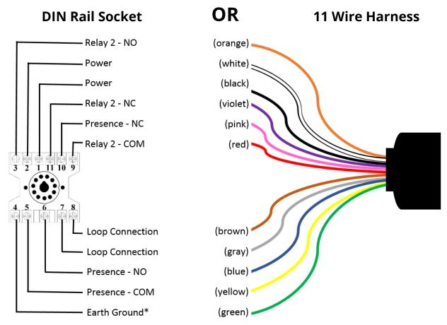
\*Must be connected to approved earth ground for surge protection to be effective
